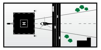
PLUSAFE unique Azimuth Guidance System for Approach (SAGA) guides the pilot with perfect precision clear of obstacles when a certain direction and azimuth angle is required by traffic control.
